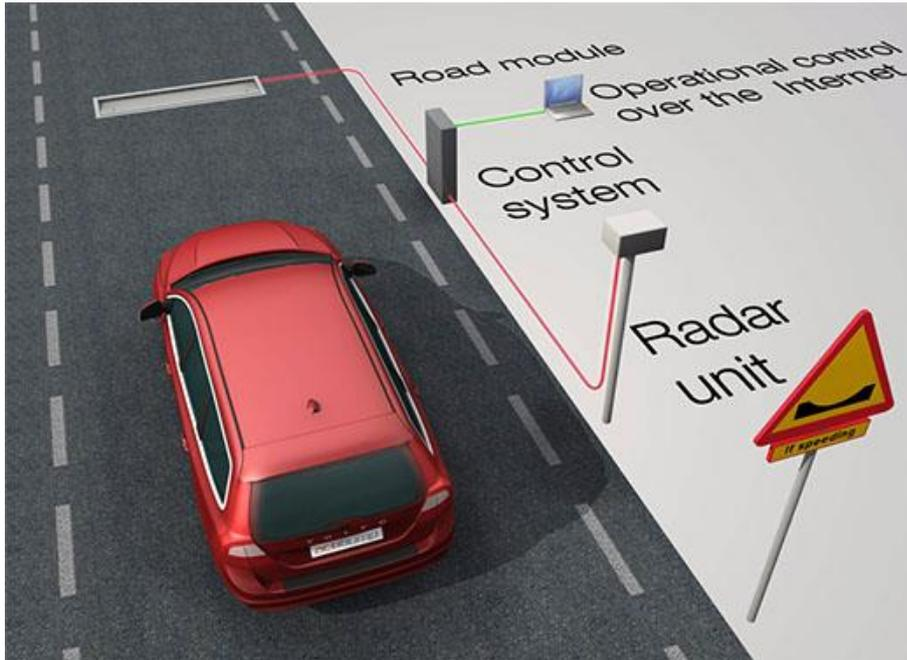
Figure 4. Technical controls of the Actibump system (Gustafson 2016, Actibump, A speed bump only for speeders, <http://www.unpressablebuttons.com/>)
