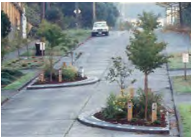
Example of a slow point (one lane) angled buildout
