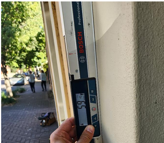
Rotation of southern wall on eastern end.
