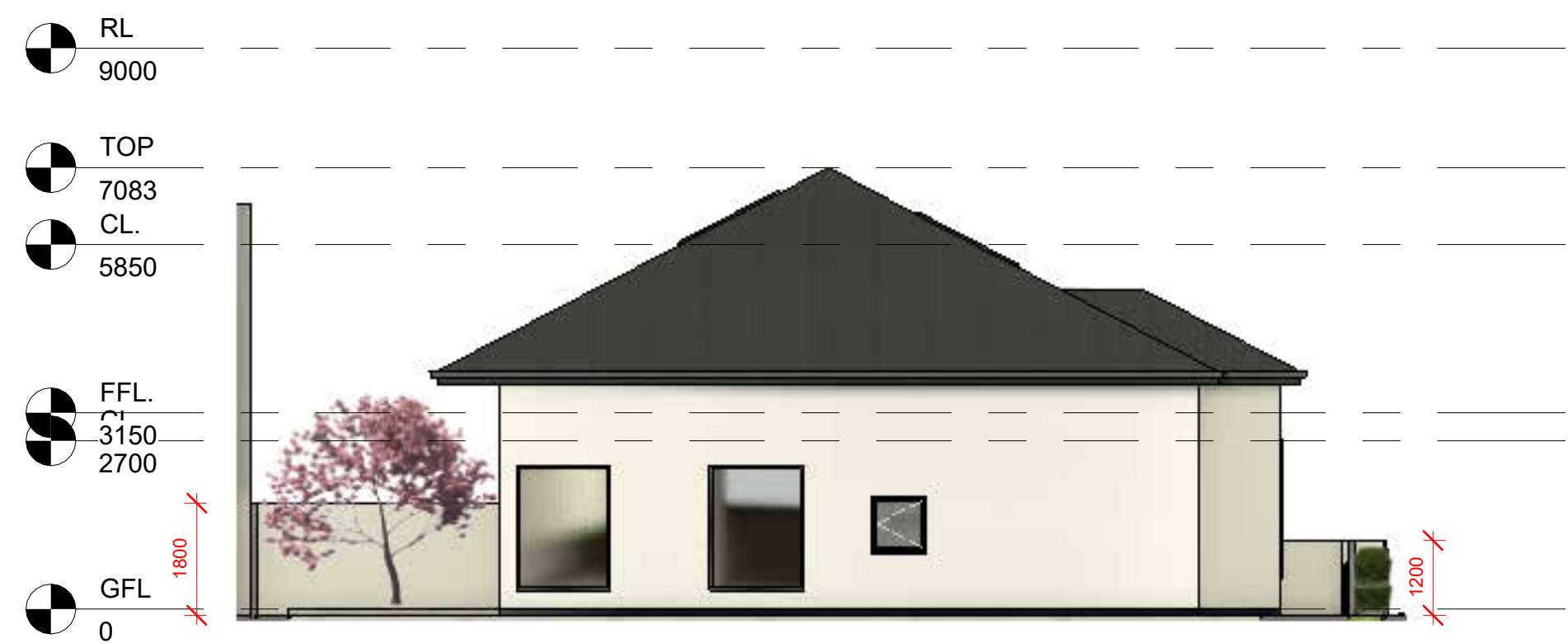
4 HOUSE B SIDE ELEVATION 1 : 100
