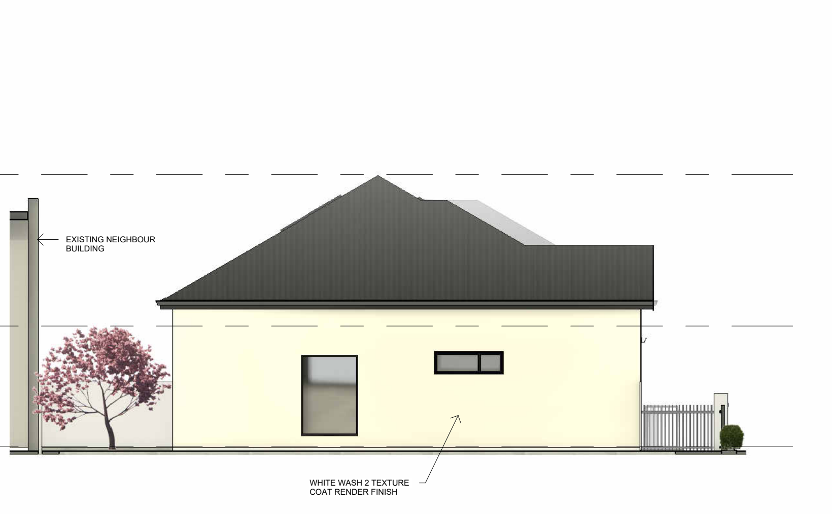
4 HOUSE B SIDE ELEVATION 1 : 100
