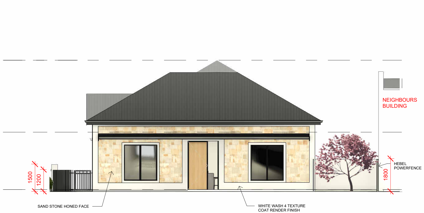
3 HOUSE A SIDE ELEVATION 1 : 100
