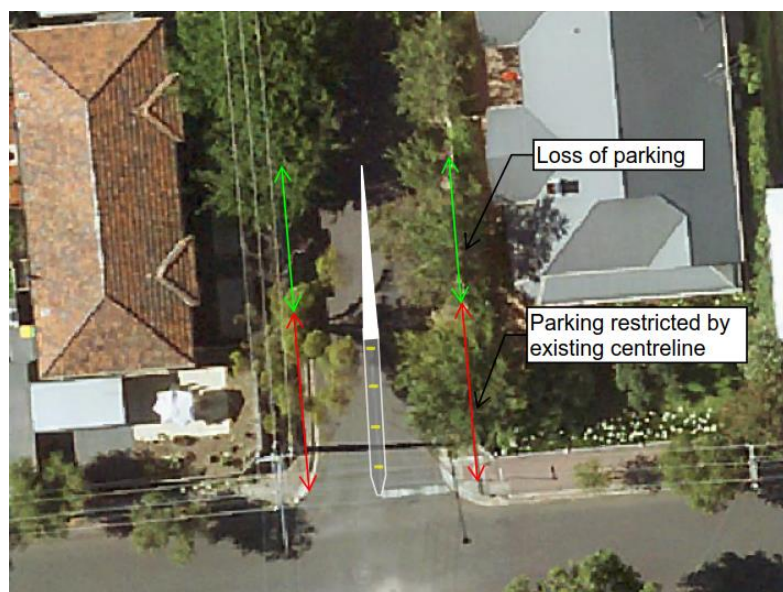
Figure 6.15 Pavement bar median on Morris Street
