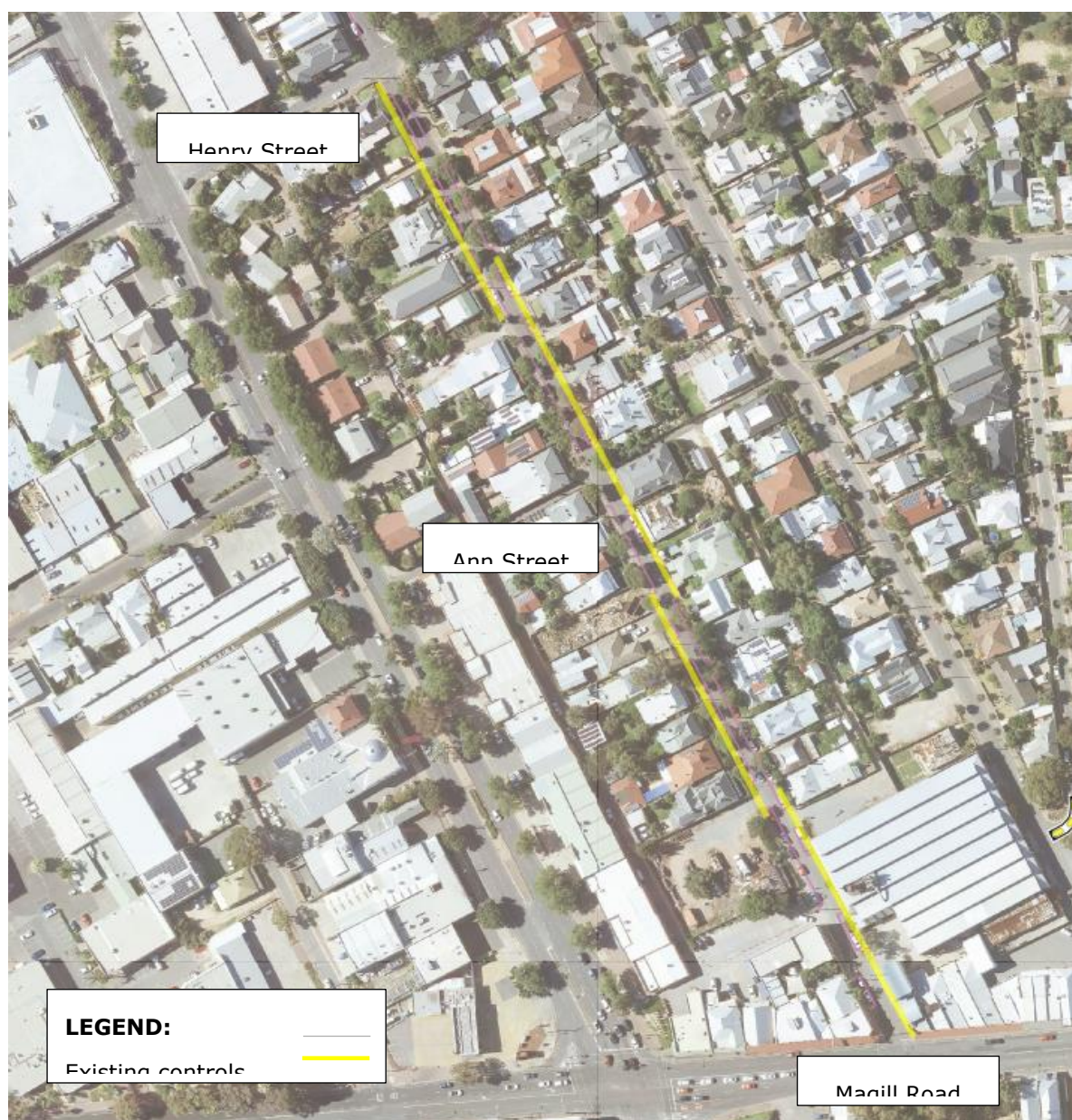
Figure 6.4 Southern end parking restrictions – Staggered
