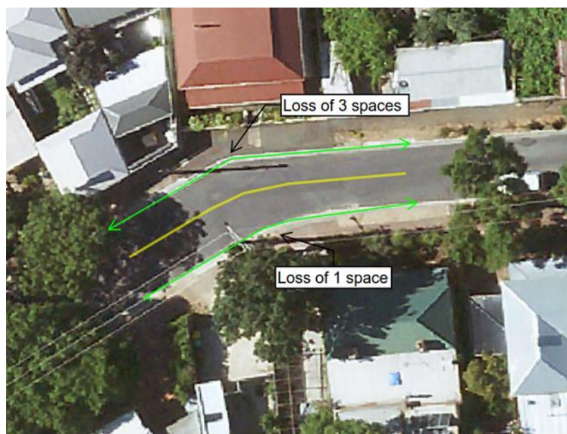
Figure 6.9 Henry Street continuous line marking
